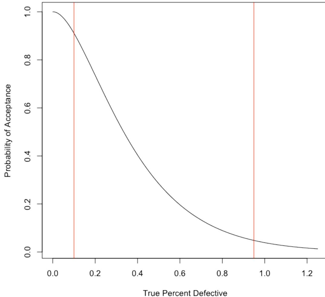
The red vertical line at the left of the OC curve is at a true percent defective of 0.1% - the chosen "Acceptable Quality Level". The corresponding probability of acceptance is 0.911. The probability that a lot with this quality level will be accepted is over 90%.
